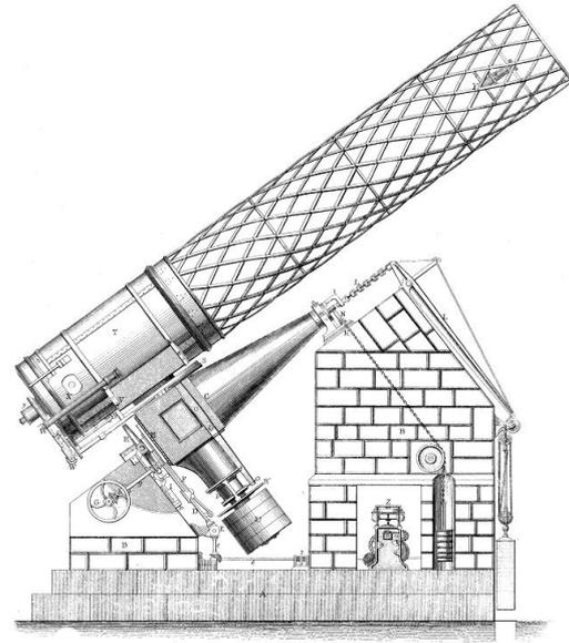
The original design drawing of the GMT by Robinson and Grubb.
