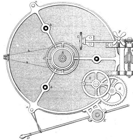
**Eyepiece end of the GMT showing the focussing wheel around the central eyepiece. The adjusting cables can be seen on the left of the focussing wheel.**
